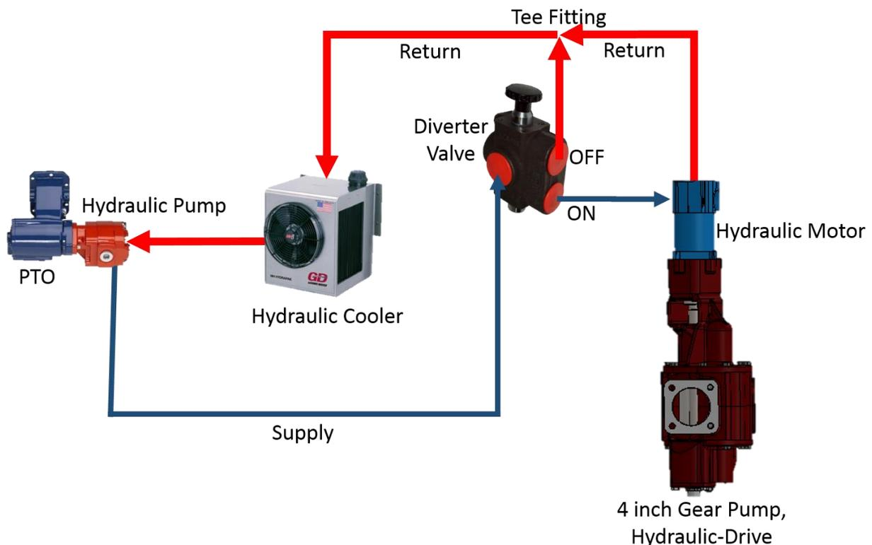
Based upon the truck transmission manufacturer and model number the PTO is selected, refer to the PTO manufacturer's technical information to select the correct PTO gear ratio that will drive the PTO shaft at 900 rpm when the truck engine is operating at 900 rpm. Then select a hydraulic pump (attaches to the PTO) and a hydraulic motor (attaches to the pump) that have a 1 to 1 ratio. If the system is already installed and not operating at the correct rpm, this
